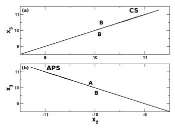
FIG. 3. Lorenz attractor: The evolution of a response system (x variable) for two different sets of initial conditions at  $\epsilon = 1.59$ , where these conditions converges to (a) the same attractor B (CS,  $x_2 = x_3$ ) I (b) either of symmetric coexisting attractors A and B (APS,  $x_2 = -x_3$ ). The parameters are those of Fig. 2(b).
