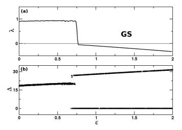
FIG. 1. Lorenz (response) system: (a) the largest conditional Lyapunov exponent (LCLE) and (b) the average synchronization error ( $\Delta$ ) between response system and its auxiliary copy, with coupling parameter  $\epsilon$ .
